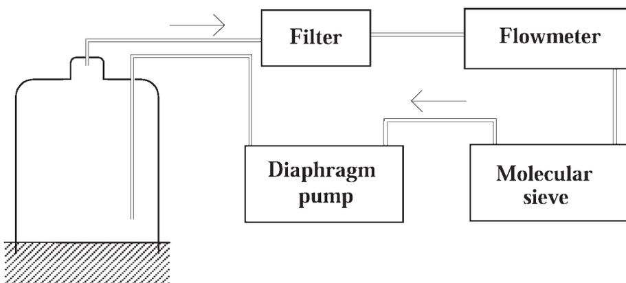
**Fig. 2.** Schematic representation of sampling system used to obtain cumulative monthly samples of soil  $\text{CO}_2$  for radiocarbon analysis
