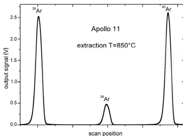
**Fig. 1.** An example of mass spectrum recorded for argon extracted from lunar regolith.
