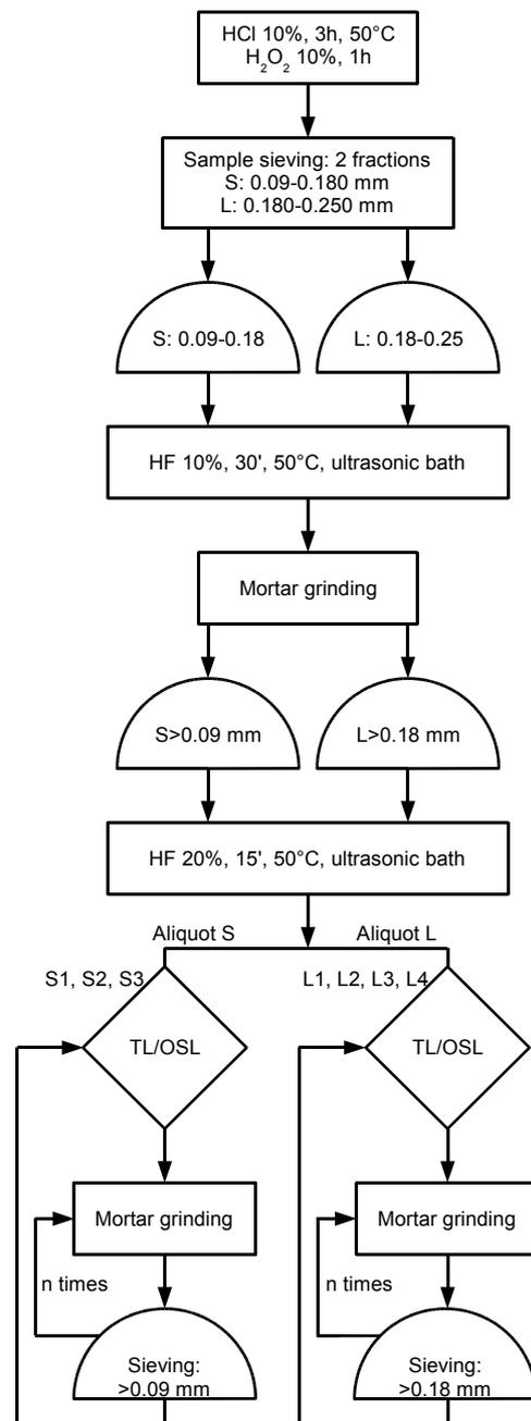
**Fig. 2.** Scheme of the sequence of chemical and mechanical treatments that the fluvial samples underwent. Each measurement of feldspar abundance is identified by a code standing for aliquot-fraction-measurement cardinal number. The number of times of each mortar/grinding/sieving sequence is stated in the Material and Methods section.
