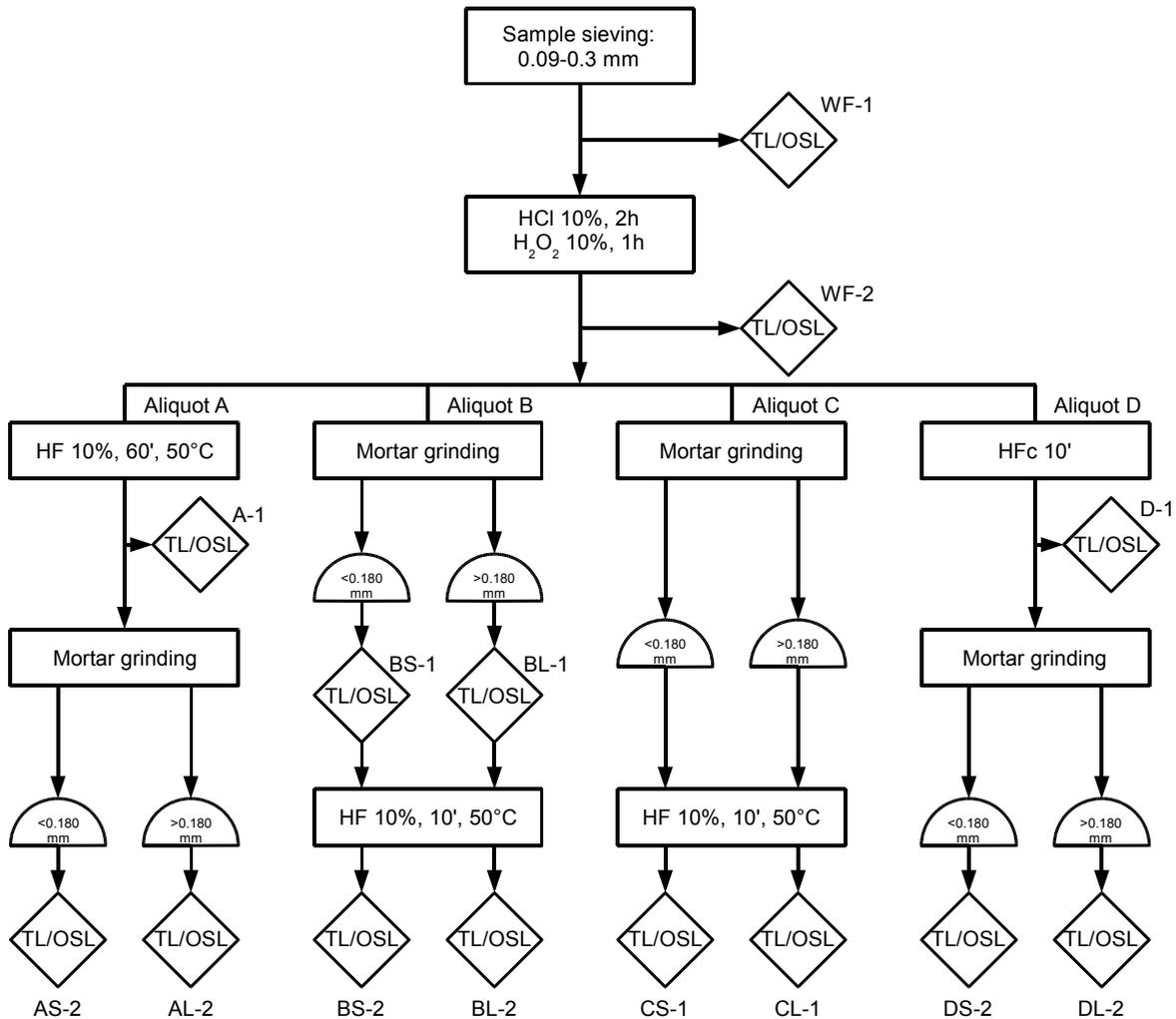
**Fig. 1.** Scheme of the sequence of chemical and mechanical treatments that the aeolian samples underwent. The mortar step consists of a single grinding of 3 seconds followed by sieving. Each measurement of feldspar abundance is identified by a code standing for aliquot-fraction-measurement cardinal number.
