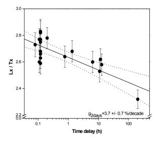
**Fig. 10.** Anomalous fading data for a representative aliquot of sample A1. Plotted are the measured  $L_i/T_i$  ratios versus the logarithm of the time elapsed since the end of the irradiation. A linear dependency can be noticed. Dotted lines indicate upper and lower 95% confidence levels.
