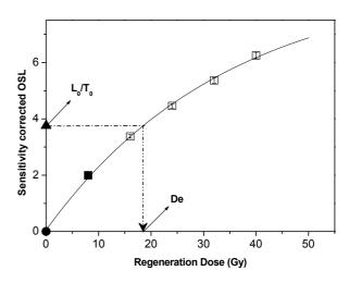
**Fig. 4.** Sensitivity corrected OSL growth curve for sample V1. Data points were fitted using a saturating exponential. Zero dose and recycling points are represented as a solid circle and solid square, respectively.
