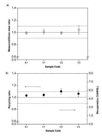
**Fig. 9.** SAR-IRSL dose recovery data for all investigated samples using polymineral fine grains. The thermal treatments consisted of 10s preheat at 220°C and cut heat to 220°C. (a) measured to given dose ratios; (b) recycling ratio and recuperation. Error bars represent 1 standard error.
