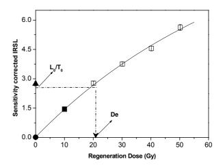
Fig. 7. Sensitivity corrected IRSL growth curve for sample A1. Data points were fitted using a saturating exponential. Zero dose and recycling points are represented as a solid circle and solid square, respectively.
