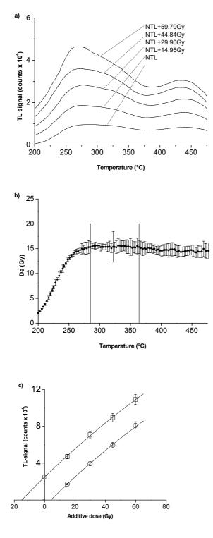
**Fig. 3.** *TL* data for sample A1; (a) *TL* additive glow curves, (b) plateau range, and (c) additive growth curve (solid squares) and second-glow growth characteristic (solid circles).
