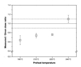
**Fig. 5.** Quartz SAR-OSL dose recovery data for sample V3 as measured to given dose ratios as a function of preheat treatment. The solid and dashed lines (eye guides) represent a measured to given dose ratio equal to unity and a 10% deviation of this ratio from unity, respectively.
