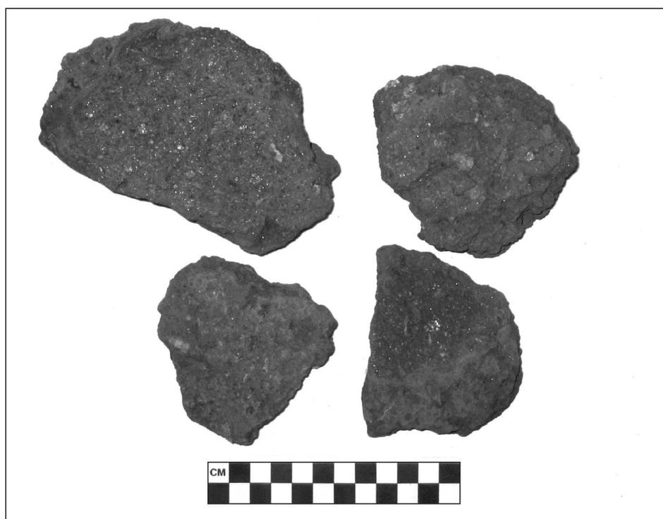
**Fig. 2.** Examples of furnace lining fragments from Kephala.
