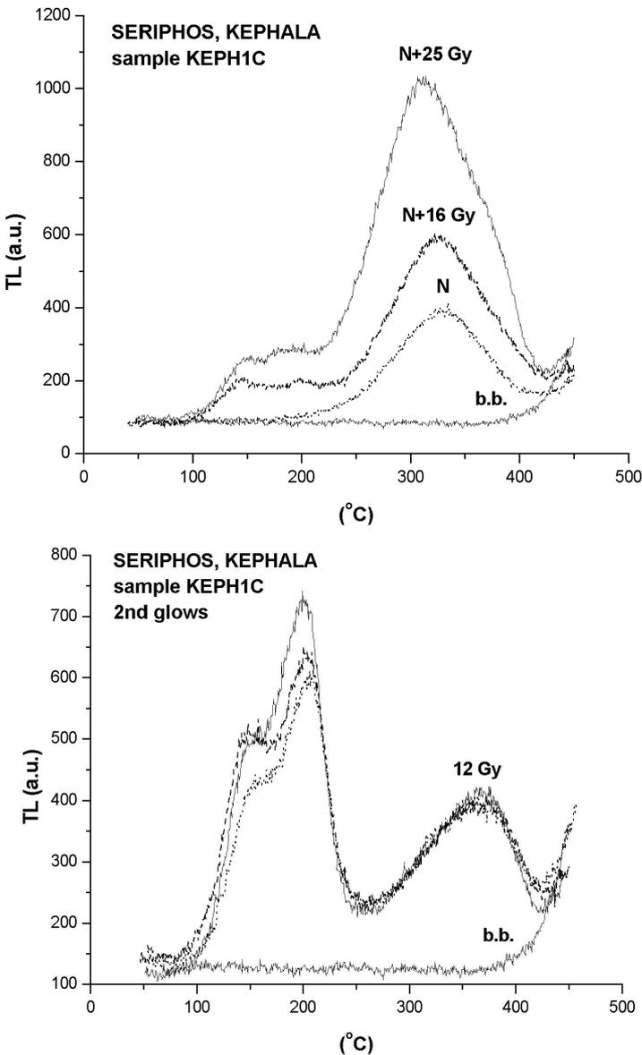
**Fig. 5.** Natural and additional irradiated glow curves for quartz aliquots of sample KEPH1C (upper plot). The 2<sup>nd</sup> glows of the same aliquots are given in the lower plot.
