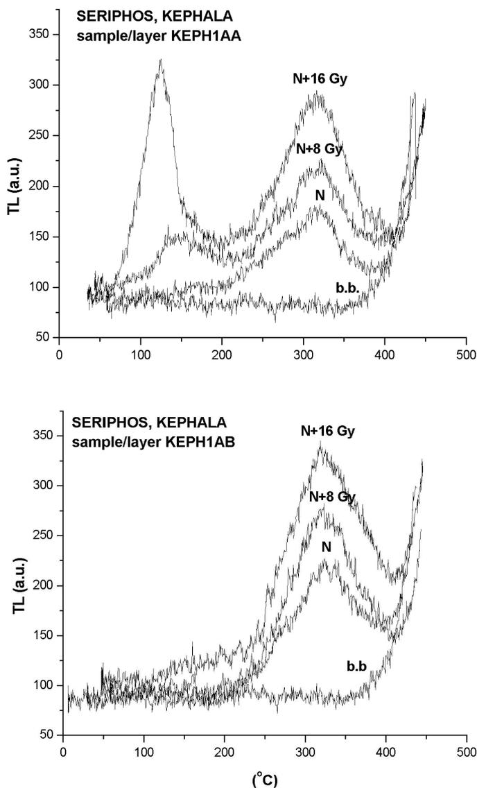
**Fig. 3.** Glow curves for quartz aliquots from the layers KEPH1AA (upper) and KEPH1AB (lower plot). The natural (N) and additional irradiated glow curves are shown. b.b. stands for the black body signal.
