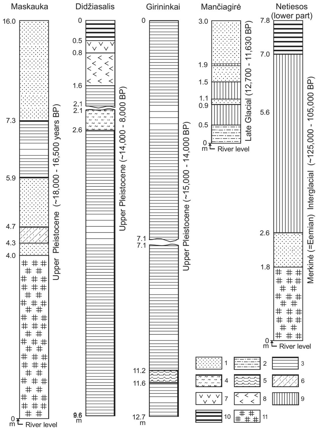
**Fig. 2.** Palaeomagnetically investigated sections: Maskauka, Didžiasalis, Mančiagirė and Netiesos. 1 – sand, 2 – silt, 3 – varved clay, 4 – homogeneous clay, 5 – clay disturbed by cryogenic process, 6 – till, 7 – limnic tufa, 8 – sapropelite, 9 – gyttja, 10 – peat, 11 – deluvium.
