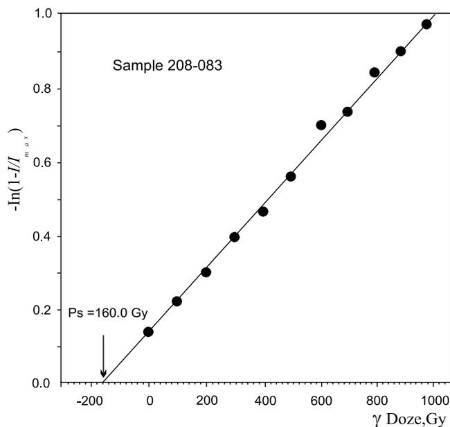
**Fig. 3.** Dose responses of the paramagnetic centres at  $g=2.0012$  in freshwater mollusc shells from the Butėnai lacustrine deposits. The solid line show the best logarithmic fit for experimental data points (circles), obtained by phase sensitive detection (PSD) technique; each point is the mean of 10 read-out values.
