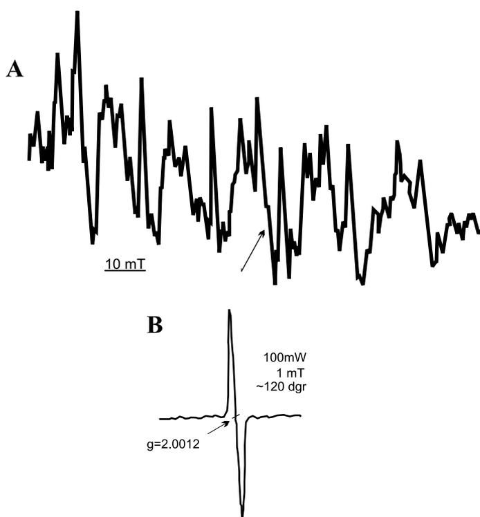
**Fig. 2.** Typical ESR-spectrum of calcite freshwater mollusc shells from Butėnai lacustrine deposits about 330 ka in age (Neravai site). Radiation-induced signal (arrow) is super-imposed by forbidden  $Mn^{+2}$  transition line (A). Analytical line at  $g=2.0012$  (B) is separated by phase sensitive detection (PSD) technique.
